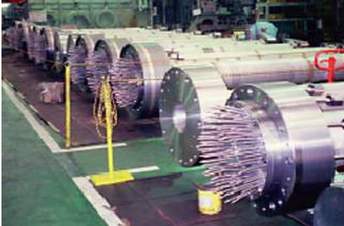
The cylinder deck (10 cylinder version): cylinder liners are die-cast ductile cast iron notice the size of the head studs!
